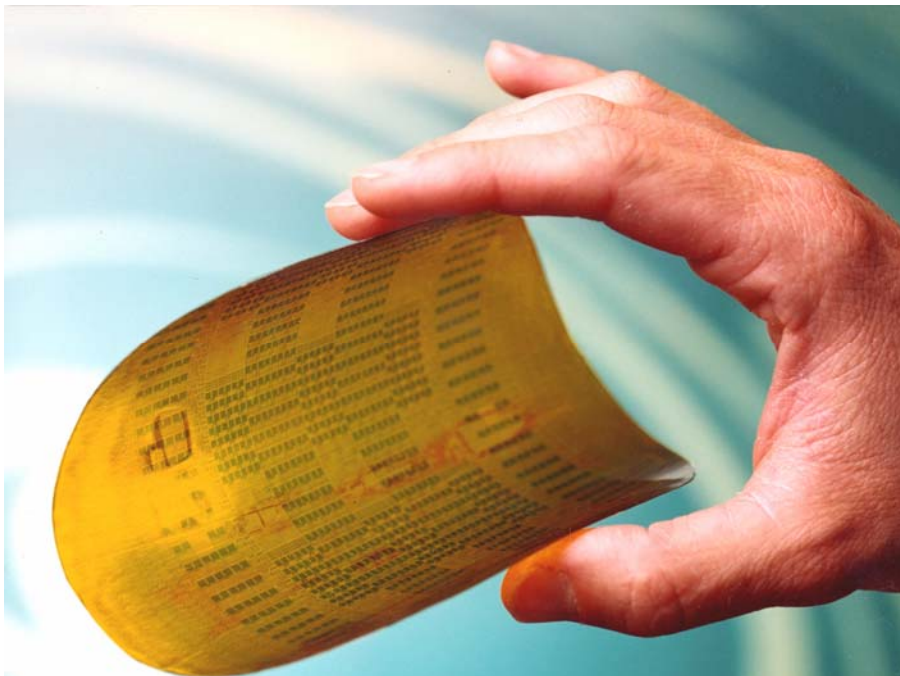
Figure 2: Organic electronic circuits on a flexible plastic foil. (Photo by Dago de Leeuw, Philips Research). In future electronic circuits can simply be printed e.g. modified inkjet printers.
